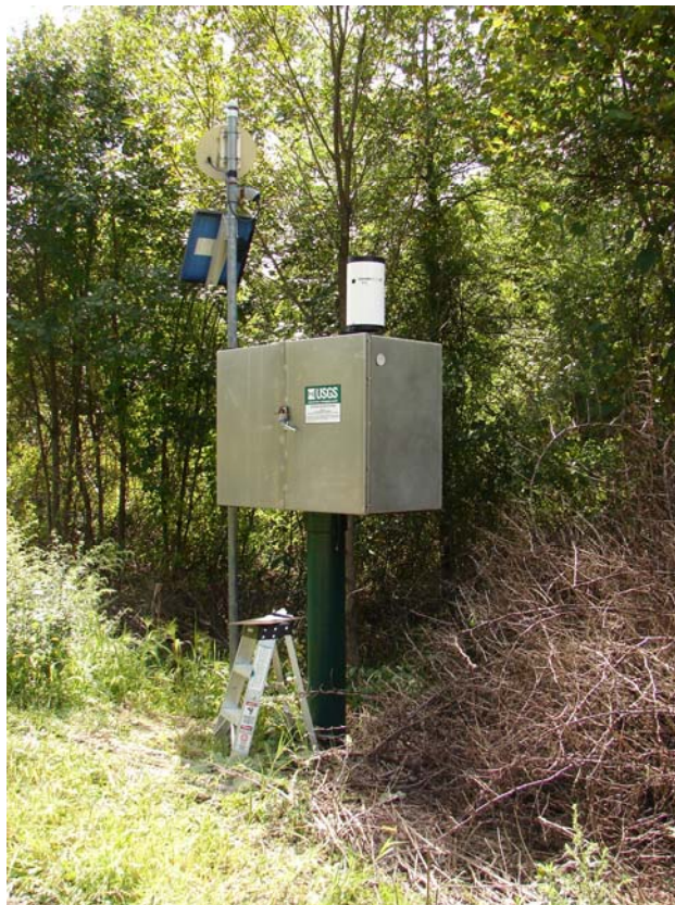
Gage on S.B. Raritan River at Four Bridges; a traffic control box raised on a pipe, above flood stage
